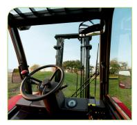
Optional fully enclosed cab with heater, defroster and air conditioning.
