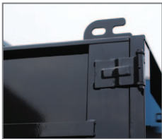
Tarp Tie Down Tension Cleats Positioned on the top of the body for easy door opening
