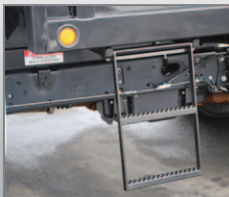
Slide Away Access Ladder Underbody self-storing ladder for easy tarp control or cab guard access
