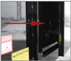
Rear Door Holdbacks Mounted on the side of the body to hold the rear door open to access the bed area
