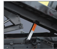
Scissor Hoist 50° angle, double-acting 8-13 ton capacity
