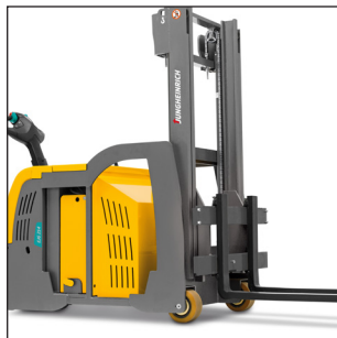
Increase in ground clearance with large load wheels
