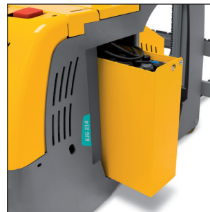
Lateral battery exchange (optional)
