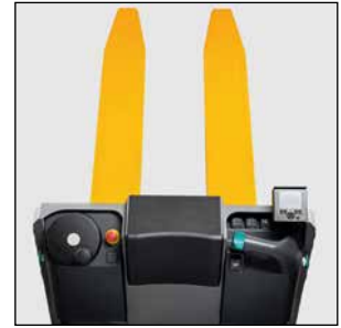
Controls and additional display in load direction
