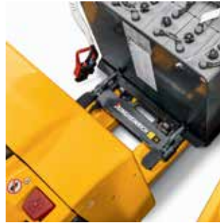
snapFIT Battery Extraction
