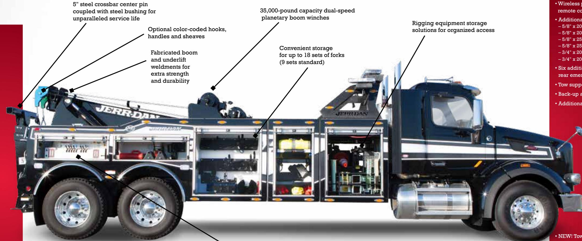
5" steel crossbar center pin coupled with steel bushing for unparalleled service life
