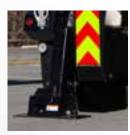
Telescoping rear stabilizers with integrated fold-down spade feet
