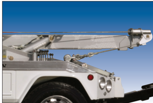
Jerr-Dan's Exclusive Self-Contained Recovery Boom is Hydraulically Actuated for Raise, Lower and Extend Functions.
