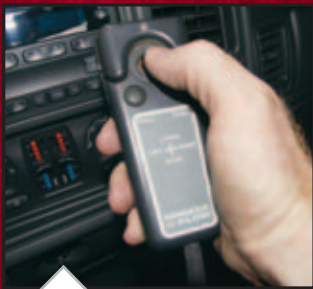
The compact joystick control puts full control of all plow functions in the palm of your hand.
