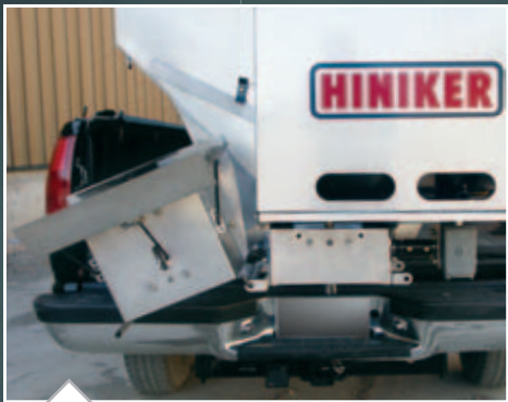
Swing-away spinner chute for easier unloading and improved trailer hitch access.
