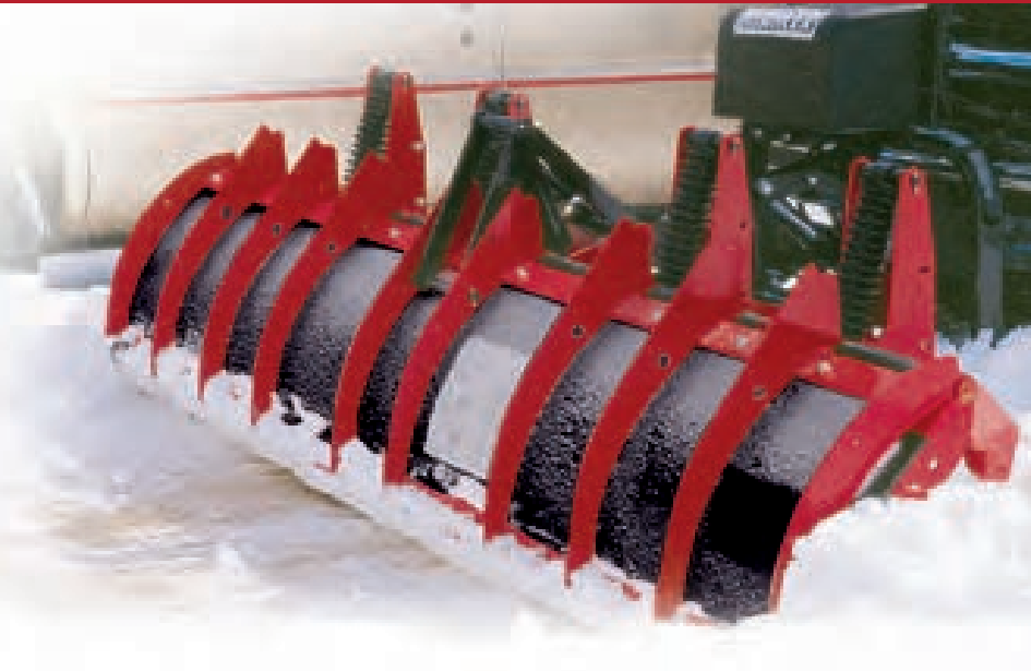
*Shown with optional box ends. *Optional box end wings reduce spillage to capture more snow.
