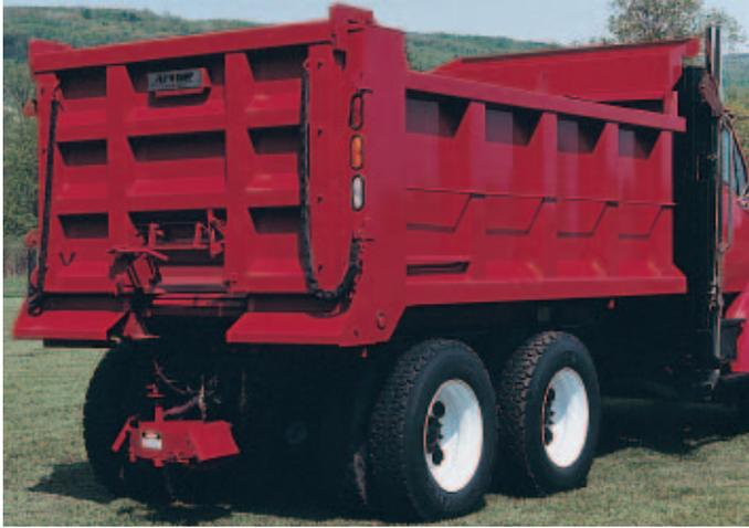
The Flo'N Dump® spreads material while the body is down on the chassis which makes for a low center of gravity and consequently a safe and stable load on icy roads.
