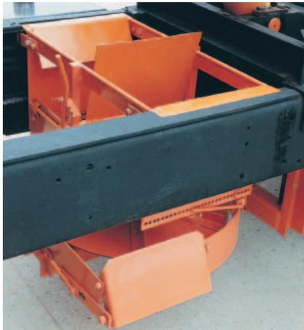
Optional Front Spread Model features exclusive chassis frame chute. This chute allows precise material applications – from spreading of all material under the truck to all material to the left lane of the truck or any combination in between.
