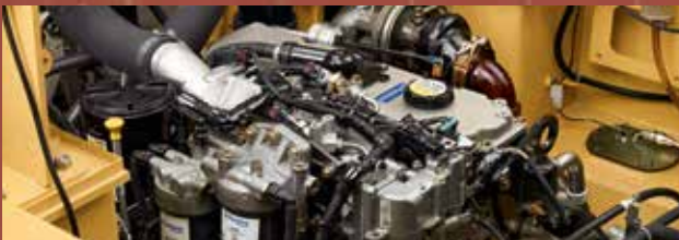
Fuel-efficient Perkins diesel engine EPA Tier 4 Final-compliant
