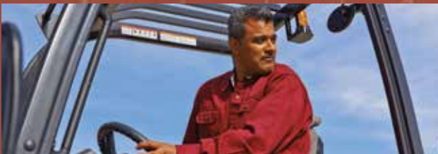
Front-to-back visibility Narrow mast channels with a large window of vision and a low profile counterweight promote good visibility while traveling
