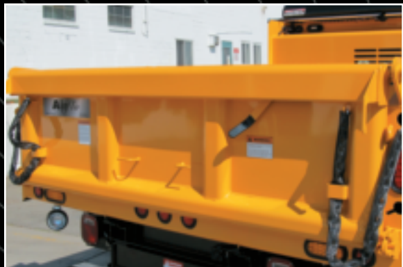
The single handle tailgate latching system allows for fast and convenient tailgate lowering.
