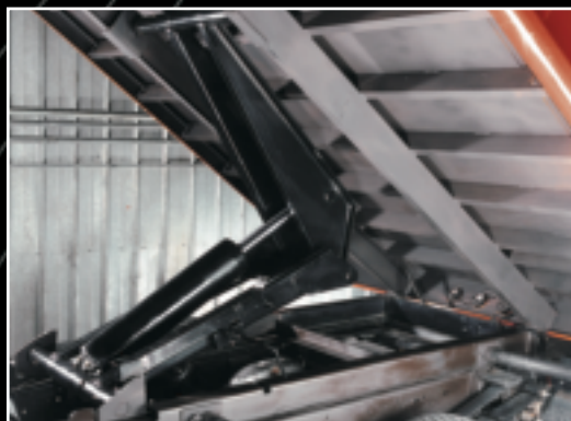
The advanced designed scissor hoist provides unmatched loadlifting power with load dumping stability. The entire floor is supported by 3" structural channel cross members on 12" centers.
