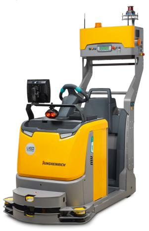
EZS 350a NA – Tow Tractor Towing capacity: up to 11,000 lb (5,000 kg)
