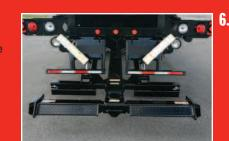
6. Optional Hydraulic Stabilizer with 4,000 lb Wheel Lift Includes No-Lube<sup>™</sup> pivot joints and 4-way receptacle for auxiliary tow lights and direct mount hydraulic counterbalance holding valves, if applicable.
