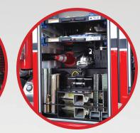
TILT-DOWN DRAWERS, TIRE LIFT, TRAFFIC CONES, CRIBBING, RATCHET, BROOM & SHOVEL STORAGE
