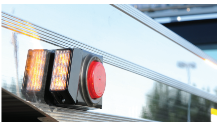
Side-mounting helps to minimize potential blockage from payloads
