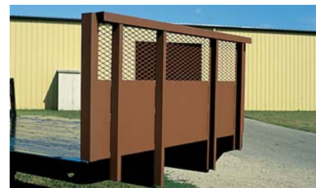
42" bulkheads with mesh windows are optional for both Fleet and Standard platforms. Fleet uses stake pockets; Standard welds to platform frame.
