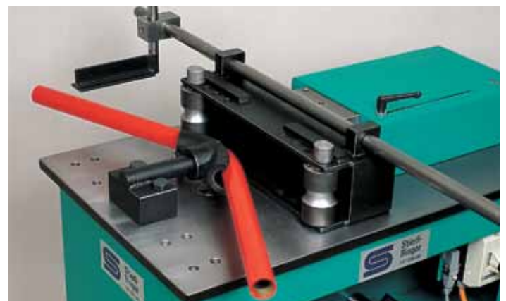
132 Gasrohrbiegen Bending of pipes
