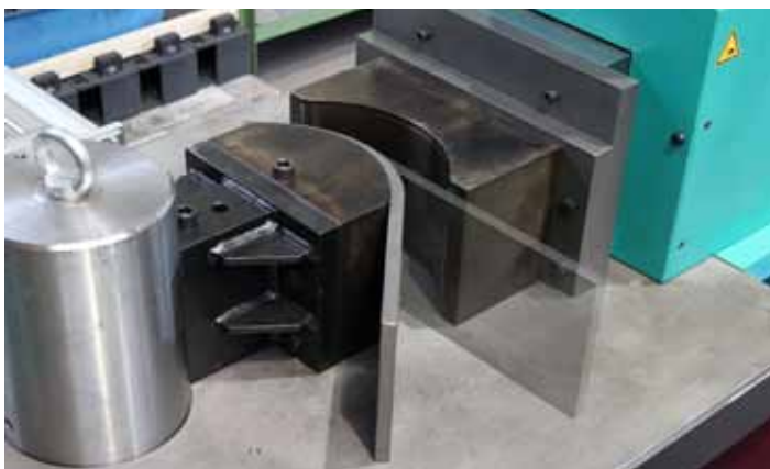
171 Pressbiegen / Formbiegen Press bending / Form bending
