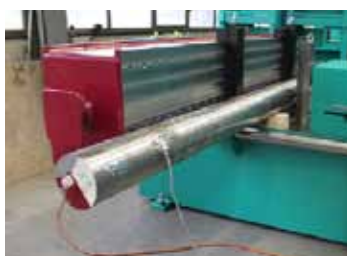
106 Richten von Rundmaterial Straightening of round material
