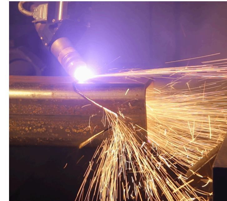
BEAM LINE AND COPING ROBOT
