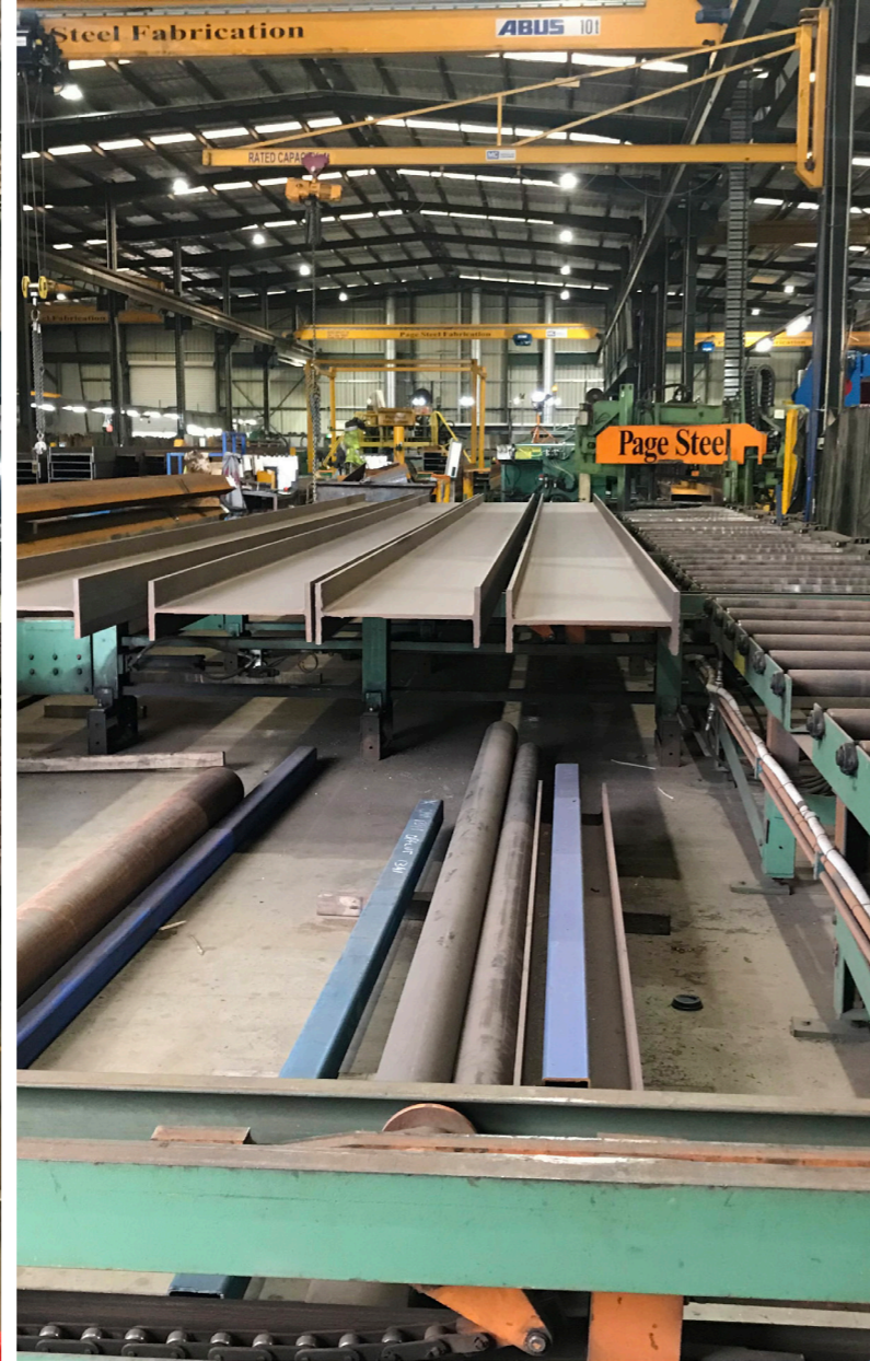
Above Left: Page Steel recently purchased a Zeman Zeman SBA single rail robotic fabrication machine, which is capable of fabricating beams 1,100mm wide and 18,000mm long.
