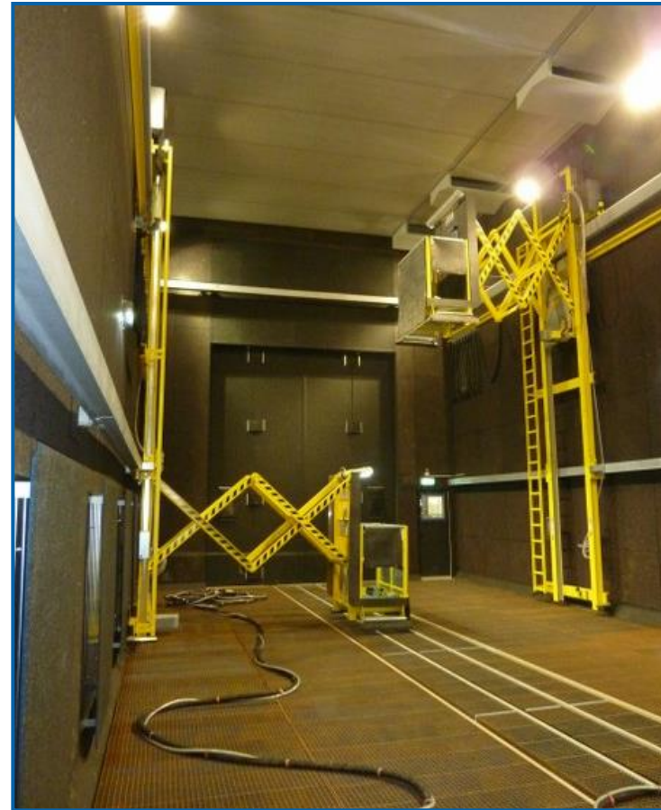
Horizontal scissor-type lifting platforms for the use in the blastroom
