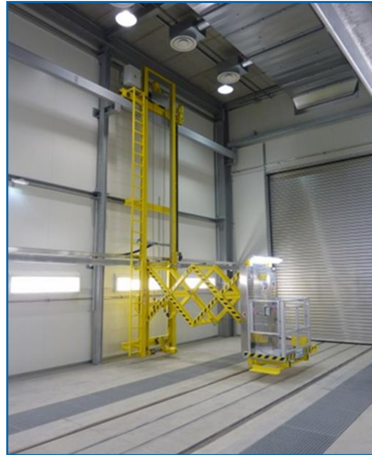
Horizontal scissor-type lifting platforms for the use in the paint spraying and preparation booths
