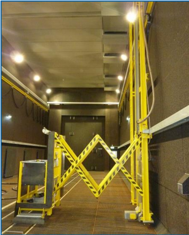
Horizontal scissor-type lifting platforms for the use in the blastroom
