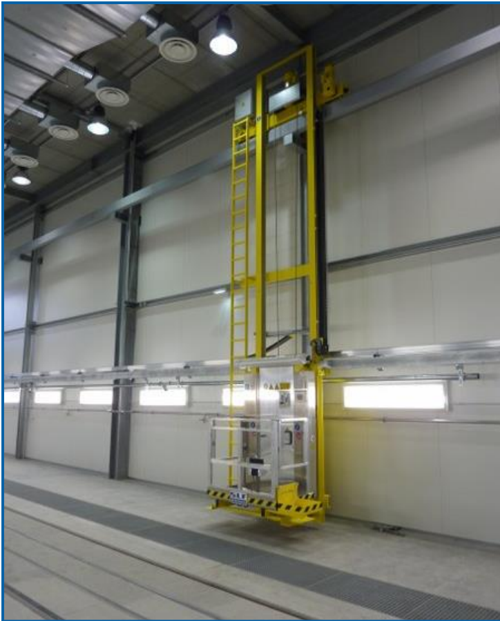
Horizontal scissor-type lifting platforms for the use in the paint spraying and preparation booths
