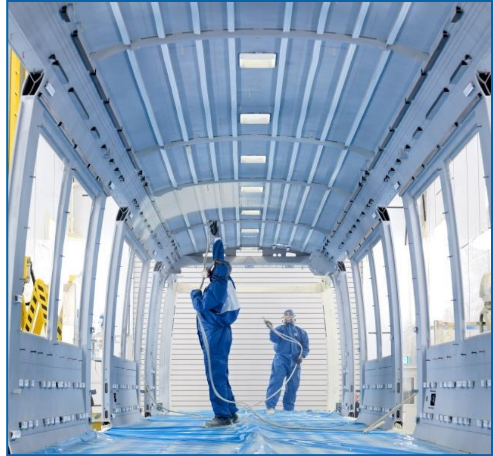
Manual paint spraying booth with horizontal scissor-type lifting platforms
