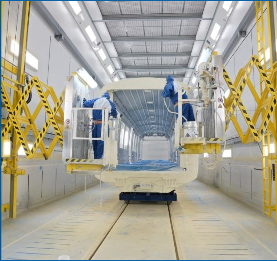
Manual paint spraying booth with horizontal scissor-type lifting platforms
