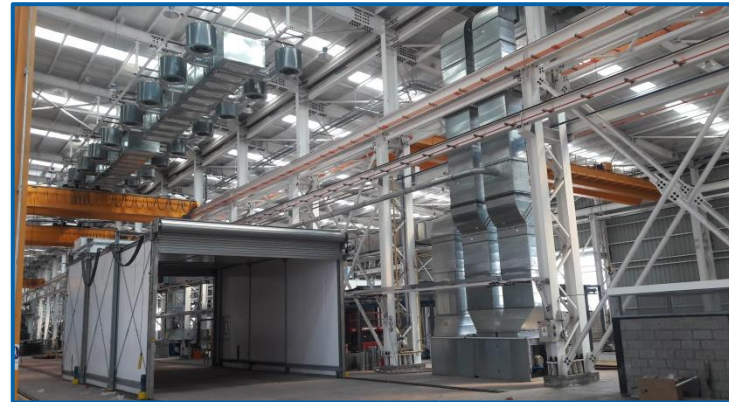
Large open-space paint spraying system with moveable telescopic dryer with three housing segments
