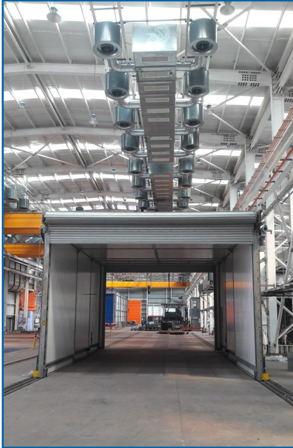
Large open-space paint spraying system with moveable telescopic dryer with three housing segments
