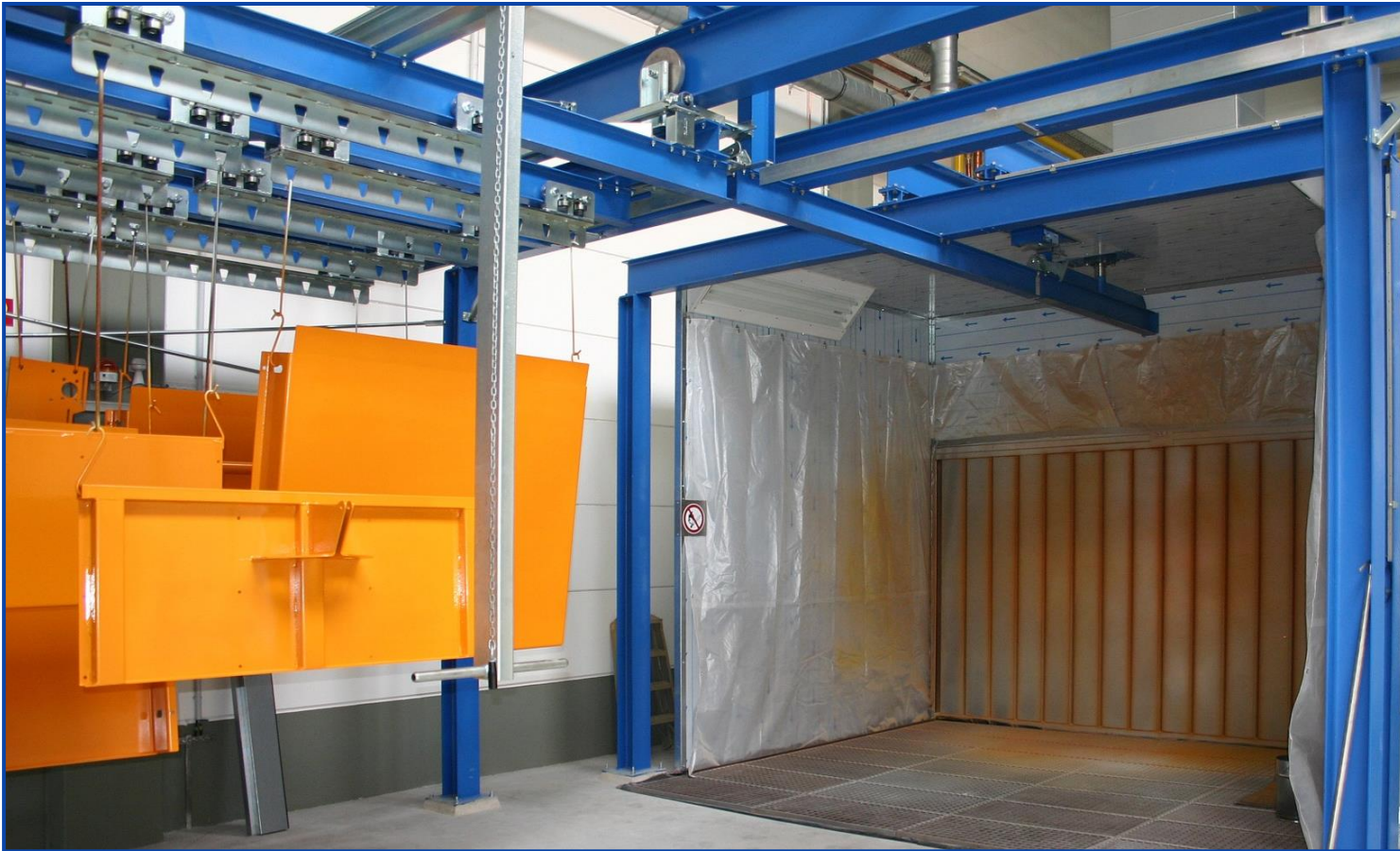
Paint spraying system for small parts consisting of manual overhead conveying system, open face spray booth, flash-off booth and dryer
