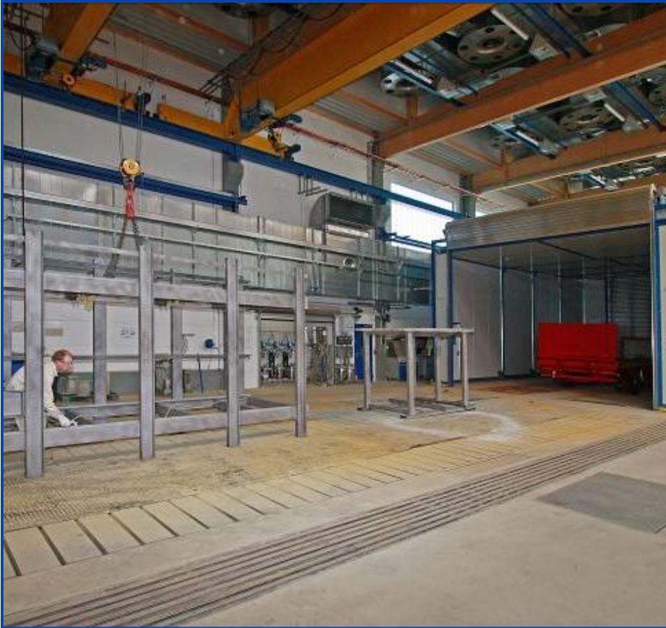
Open-space paint spraying system with movable telescopic dryer for alternating, simultaneous paint spraying and drying on both areas
