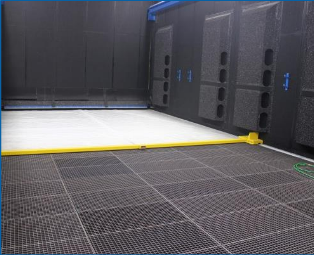
Roll-up device for the foil to cover the gratings
