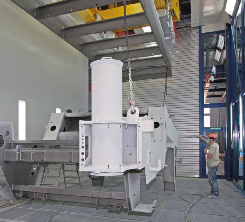
Large-volume powder coating booth for components of utility vehicles
