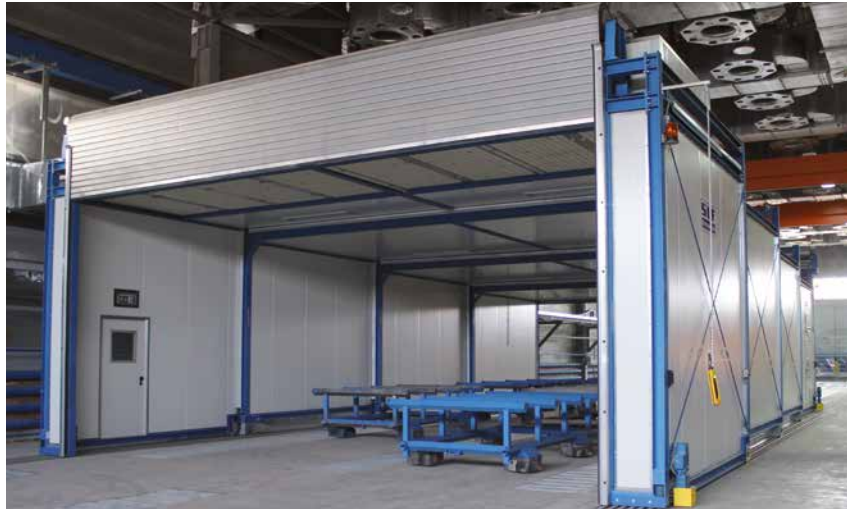
Movable and telescopic dryer with open-space paint spraying system
