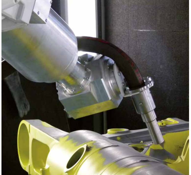
Blastroom with ReCo-Blaster® for the paint stripping of landing gears with plastic abrasive
