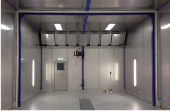
Telescopic cleaning booth in stainless steel version
