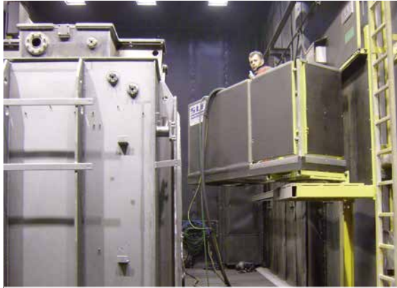
Swivelling lifting platform in a blastroom
