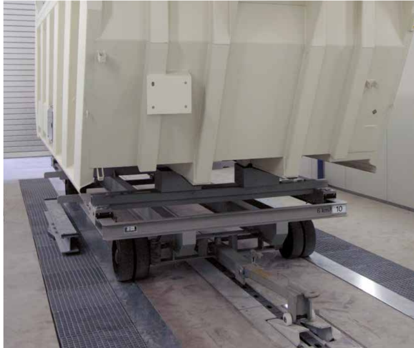
Work piece transport trolley connected to the chain conveyor in the floor of the paint spraying booth.
