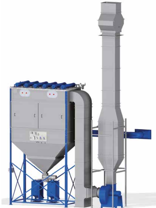
Schematic view of a dust collector with limestone powder dosing for a zinc spraying system
