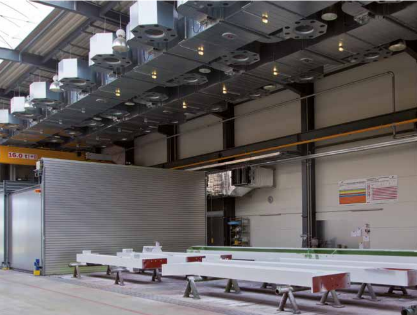
Open-space paint spraying system for steel components and steel structures
