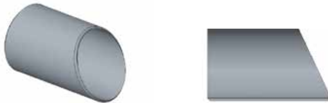
STRAIGHT CUT / MITER CUT
