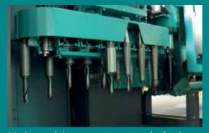
14-place tool changer on up to two axles for shorter set-up times.
