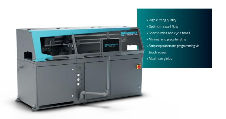
You can leave the **KKS 461 NA** unattended. This automatic mitre saw for profiles and solid materials is able to execute the tasks by itself. Highly precise material supply is effected by means of a servo motor and screw ball. Cutting speed and feed rate are calculated automatically. Ask our experts for a professional sawing advice.
