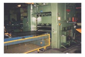
On custom order, or in case the ratio between max wallthickness and min wall-thickness exceeds 2 to 4 RI can also be equipped with additional supported lower straightening rolls and even upper supported straightening rolls. This allows a tighter straightening geometry but causes an increase of necessary straightening forces.
