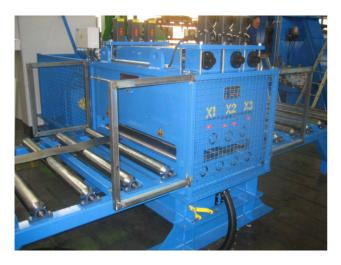
Adjustment of the straightening rollers can be done in three different modes (modes No 2 and No 3 are optional):
