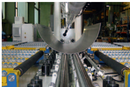
6 m bending machine for heavy plates with automatic deflection compensation.
