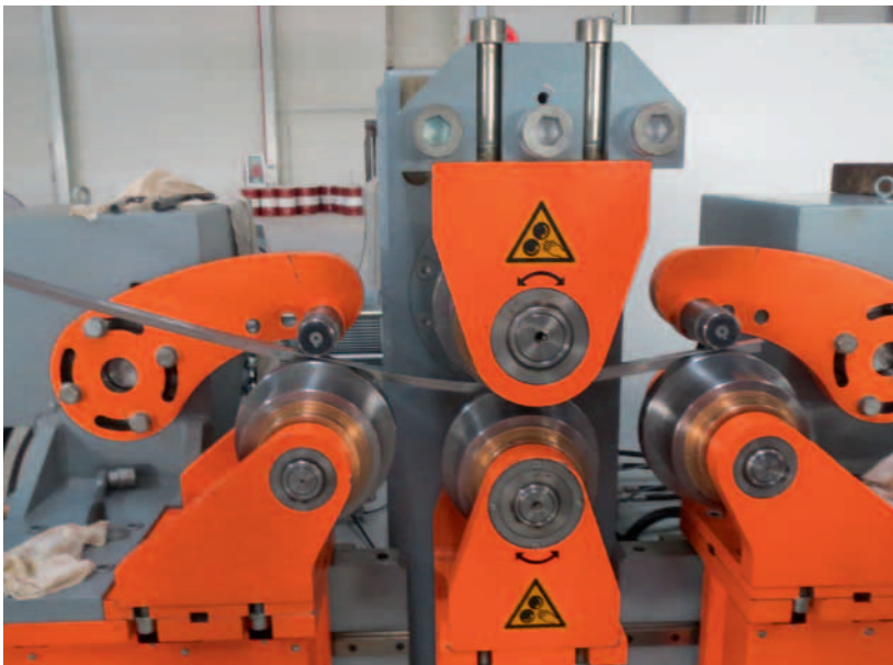
Model PRV for continuous forming of sections in all directions.
