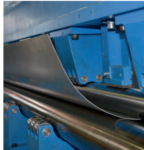
Model FKB for a max. length of 10 m. With quick changeable Top Roll and Changing Device.
