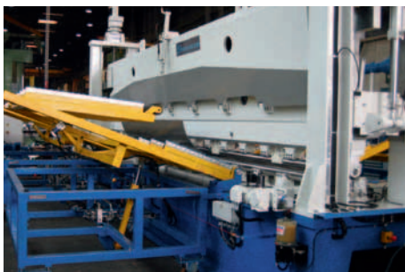
6 m bending machine for heavy plates with automatic deflection compensation.
