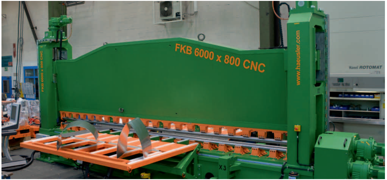
Model FKB for wall thickness up to 15 mm.
