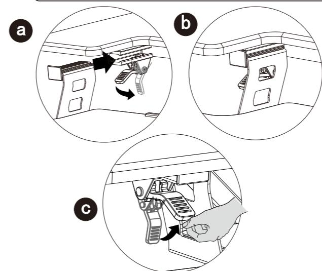
When removing the keyboard tray, release the levers completely before removing the keyboard tray.
