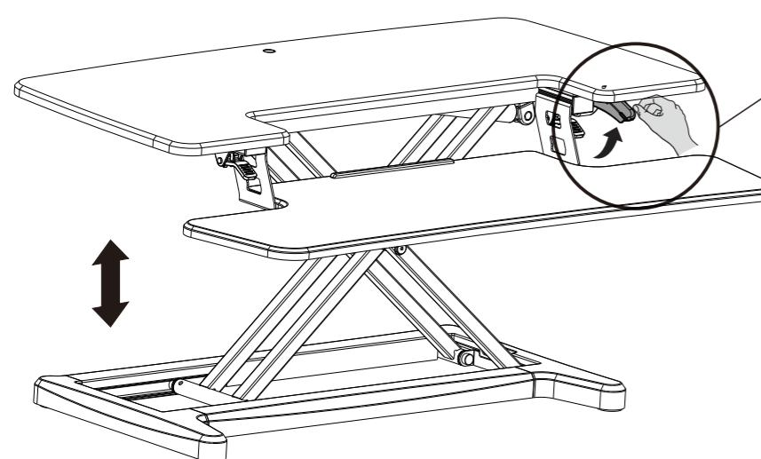
To set your preferred height, press the lever on the right side, and adjust the desk converter to the proper height.
