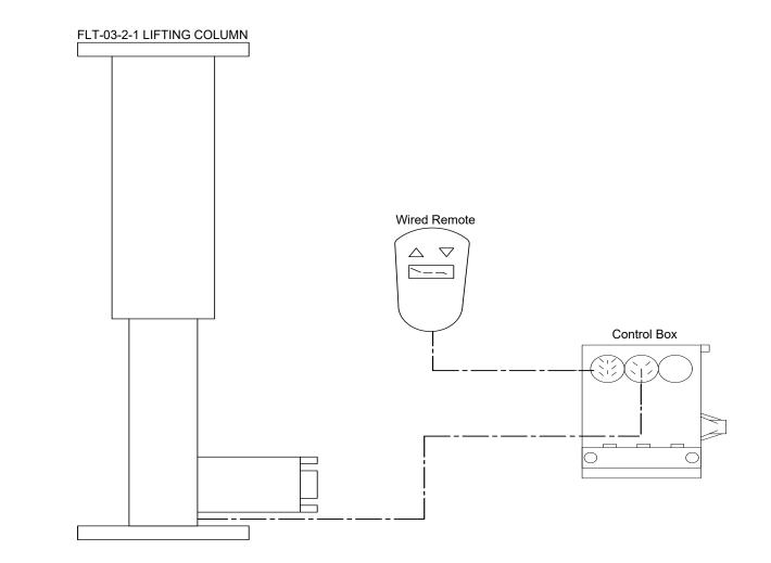
Once the table lift is installed, use the wired remote for full up and down motion control. The momentary buttons require the user to press and hold the button for both up and down control. Once the button is released, the FLT-03-2-1 will stop moving.
