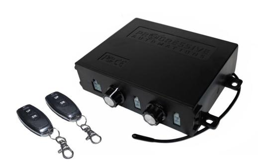
Multiple Actuators **Control Ability** 12VDC **Input Voltage** 12VDC **Output Power** Current 15A (Each Channel) Kit Includes 2 Hand Remotes, 2 Actuator Wire Harnesses, 1 Power wire Harness, 1 Control Box, Batteries **Remote Functions** Up, Down, Pause (Momentary & Non-Momentary) **Remote Battery Type** 2x CR2016 3V Lithium Cell Size (L x H x W) 5.9" x 1.3" x 3.9" 1.10 lbs Weight 18 Months Warranty
