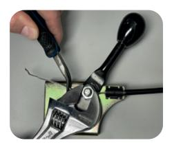
2. Carefully adjust where the cable wire is held in place. A useful starting point can be somewhere in the middle of its range. Use pliers to grab the wire if necessary. Only a small amount of force is required to move the wire to a desired location.
