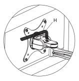
Adjust the tilt of the monitor using the provided 5X5 Allen Key (H)
