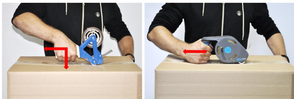
Figure 5: Representation of different coupling methods when using the standard dispenser. Red arrows indicate the corresponding directions of force.
