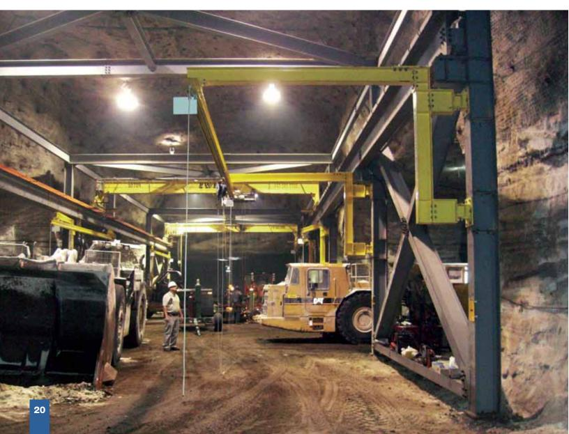
Jib Arm Systems are ideal for crane bay applications where fall protection is needed but could cause interference with day to day crane operations. The articulating feature allows the systems to be moved out of the way when not in use. The rigid style of these systems also reduces total fall distance.
