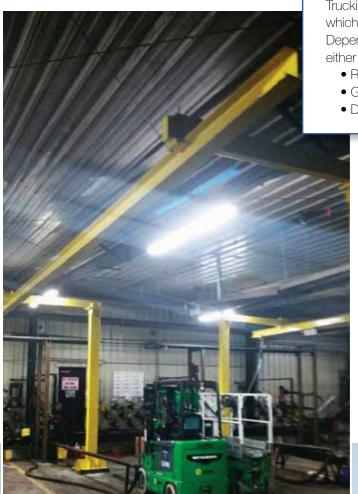
Gallows systems are used most often in outdoor applications that work with Trucking and Rail. Gallows systems always utilize overhead fall protection which reduces the fall distance since the anchorage is above the worker. Depending on the level of the working surface, gallows systems can be either rigid or lifeline systems.
