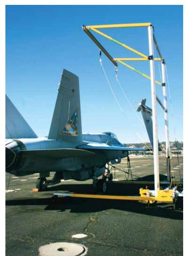
The Transportable Fall Protection offers fall protection solutions where a permanent system is simply not possible. Used indoor and outdoor in the field on mobile equipment, there are many different styles to meet your specific needs.
