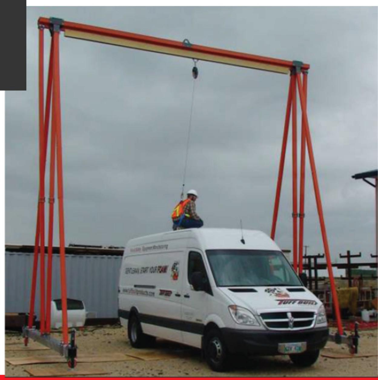
Tuff Built Product's mobile Quad-Frame allows you to place overhead anchor points where you need them in your work place. Quad or Box Frame Fall Arrest Systems are rigid rail systems built to accommodate a specific area or piece of equipment and can be designed as permanent or portable frames, for ease of relocation.
