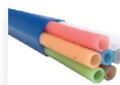
Microduct - Direct Buried, Direct Installed Duct Example ) 14/10mm 7way + Micro cable 144 Core * 7 tubes (1,008 Core) 16/12mm 7way X Micro cable 432 core * 7 tubes ( 3,024 core)
