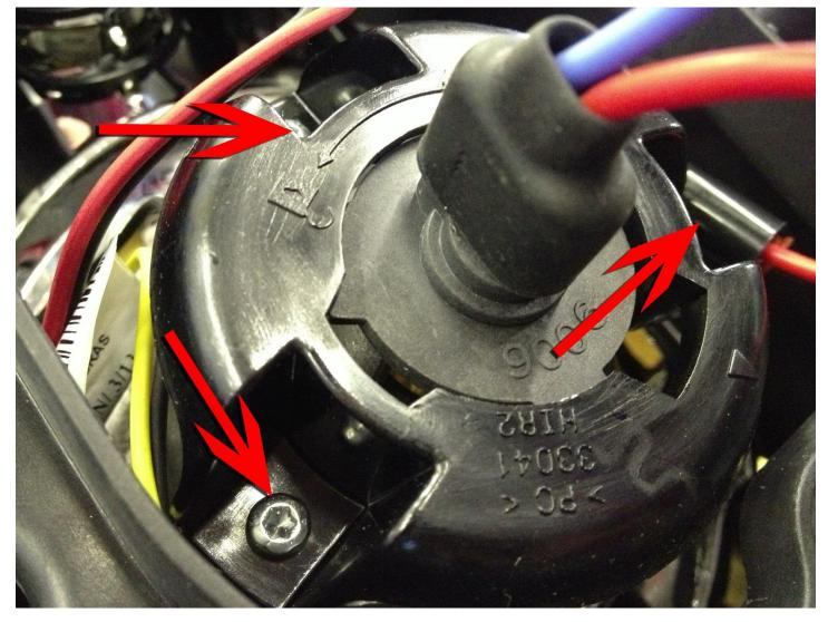
The low beam headlight bulb retainer is made of black plastic and is held onto the back side of the projector with 3 torx bit screws. If you loosen them about half way (don't have to totally remove them!) it will give you the slack needed to slide the new 9006 bulb in place without modifying it.
