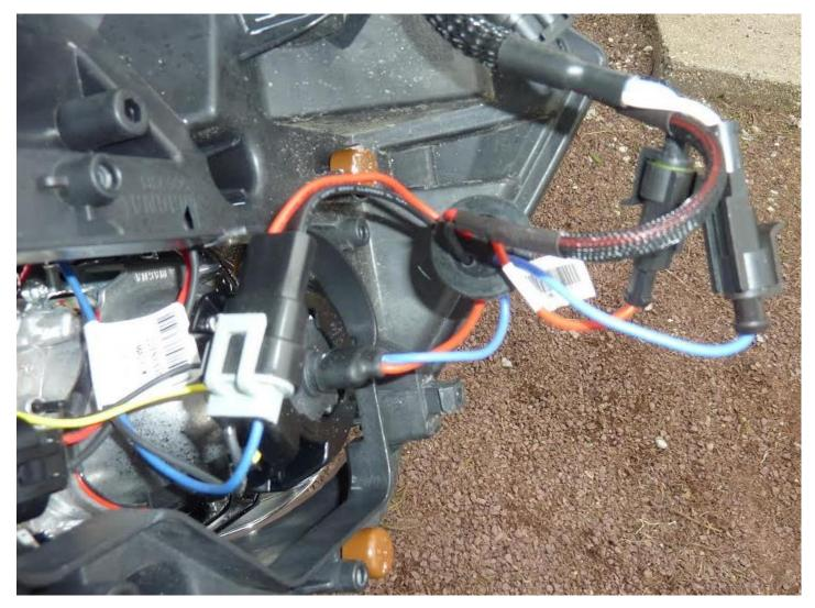
In this picture you can see the black plastic connector that holds the red and black wires is connected to the blue and black wires that used to connect to the original 9012 headlight bulb. You can also see the red and blue wires that come out of the new HID bulb pass through the rubber grommet with the other wires and go to the ballast.
