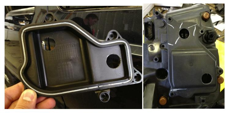
If you are just doing the low beam or just doing the high beam you'll only need to drill one hole. If you're doing both high beam and low beam you'll need to put one hole in each dust cover. You'll use these holes next to run the wiring through.
