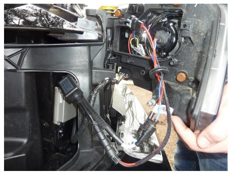
Connect the red and black wires to the black plastic 2-pin connector on the ballast, that's your power input to the ballast.
