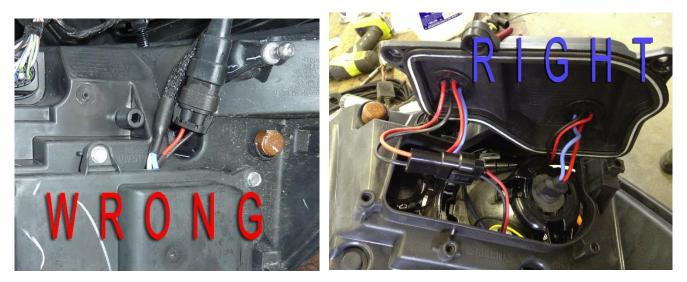
The HID bulb has 4 wires attached to it within the harness. A red and blue set of wires and a red and black set of wires. The red and black wires connect to the factory headlight wiring. The red and blue wires connect to the new HID ballast:
