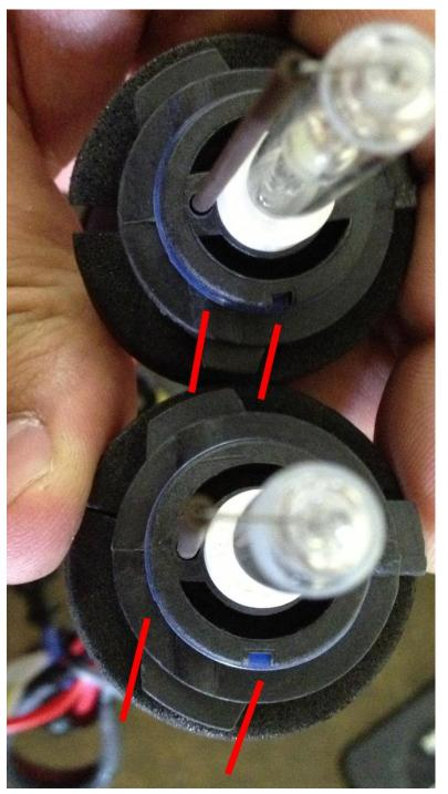
Compare the stock 9012 bulbs with the new 9006 HID bulbs and you'll see this tab is the only difference. Take a file, a sharp side cutter or a Dremel tool and carefully trim the bottom half of the locking tab off, it's the one to the right of the ceramic wire insulator that goes up the side of the glass bulb. Just keep trimming it a little at a time until it fits easily.
