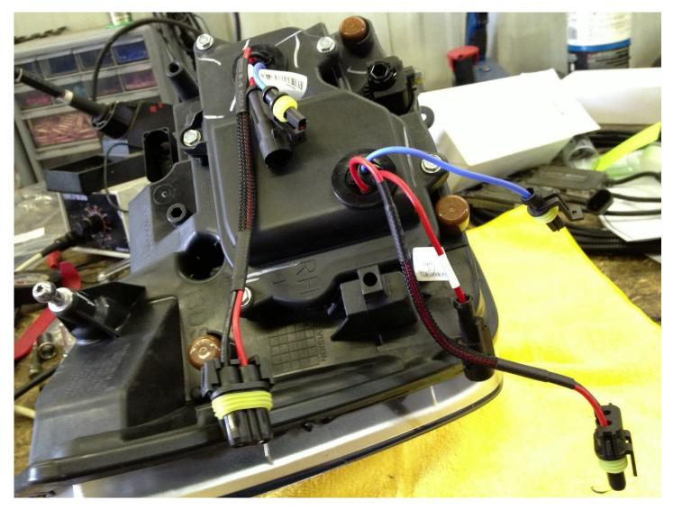
At this point all you should have to do is re-install the headlight and hook up all the wiring. Make sure you don't get the high beam and low beam HID wires mixed up, otherwise the wrong lights will turn on at the wrong time.
