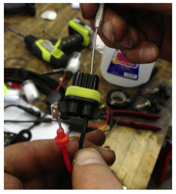
Once you have the 2 pins out you can feed all 4 wires through the hole in the dust cover and place the protective grommet in place:
