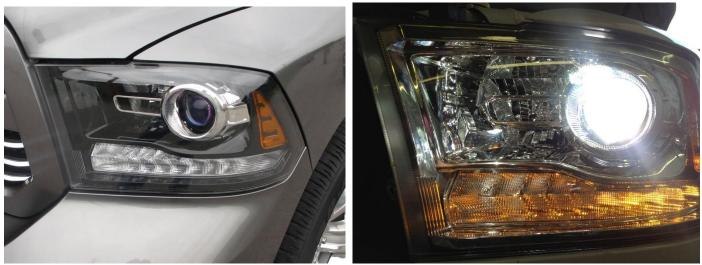
These new headlights use what is called a 9012 or 9012LL halogen bulb and although it looks like a standard halogen incandescent bulb, technically it is called "HIR" or "Halogen Infra-Red". Even though it's a new type of halogen bulb, most Ram owners still say they are terrible and should be brighter. Doing an HID conversion kit in the new Ram trucks is safe, doesn't void warranty, and is how the truck should have come from the factory, as long as you use the right parts!
