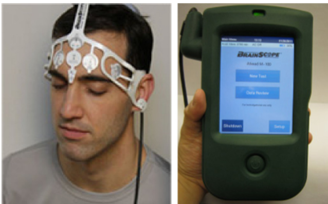
Fig. 1. A patient with the headset for placement of the electrodes in the required standard sites is shown. Hand held EEG data acquisition device is also shown.
