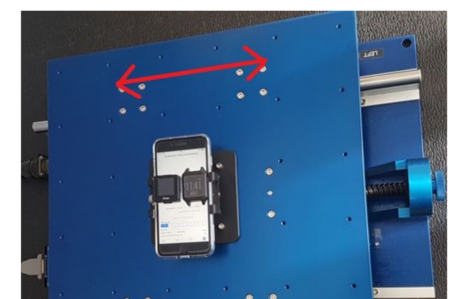
Figure 1. Shake Table with the 3 devices attached. Arrow indicates direction of movement.
