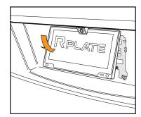
Slide Rplate onto the bracket. Slots on the back of Rplate should engage tabs on top edge of bracket.
