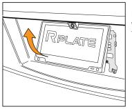
Pull out Rplate bottom while lifting off bracket tabs.
