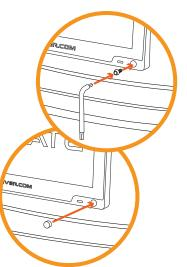
Secure the bottom of the Rplate reusing screws and grommets removed in step 1.
