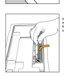
Insert fresh battery into housing while carefully folding cables/connector under the battery.
