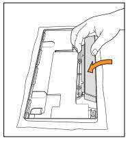
Insert metal cover tabs into housing slots and carefully push cover over battery to align screw holes.
