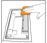
Place Rplate on a flat surface with a protective cloth between the Rplate and surface.
