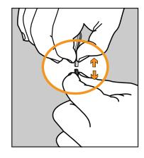
To disconnect the battery gently depress the black connector release and remove the white battery connector.
