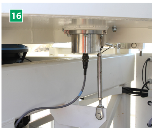
16 Moisture measurement (optional) 1 x electronic control module for connection of moisture sensor. Connection of the humidity sensors to the control.
