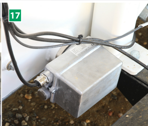
17 Water heater (optional) Electric heating in the water tank for frost protection. Complete with thermostat and switch in control cabinet for automatic operation and frost protection. Power 4 kW. Voltage 3 x 400 volts, 50 Hz.
