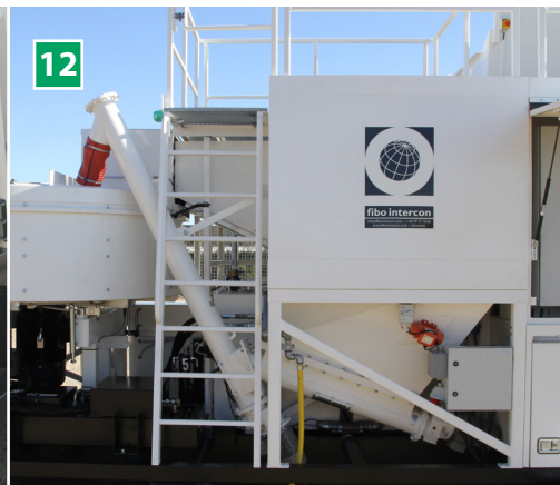
12 Cement container 2.0 m 3 (optional) The cement funnel is equipped with full and empty detectors. The opening (1x1m) is intended for big bags. Seals for dust and moisture. A vibrator on the sidewall ensures that the material slips continuously.
