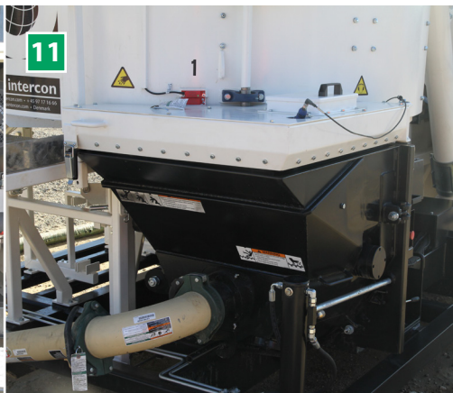
11 Concrete pump (optional) The concrete pump is a stamp pump that is hydraulically controlled. Storage tank with full indicator, safety cover and a safety switch for cleaning. Storage tank approx 400 litres. Capacity 10 m 3 / hour. Conveyor distance max. 25 m.
