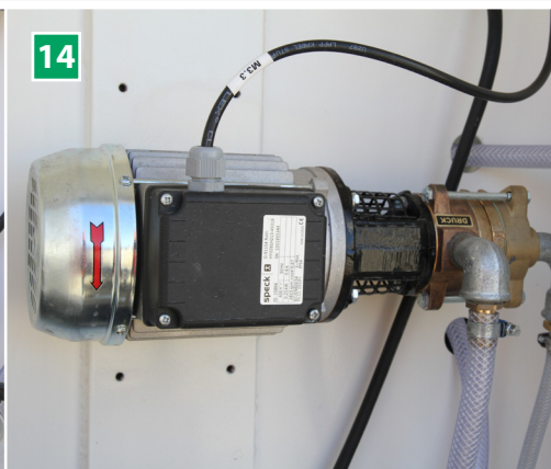
14 Chemistry pump (optional) Dosing pump with 0.25 kW for additives. 3/8" suction hose, check valve and stainless steel strainer. Possibility for installation of 1 - 4 additive pumps.
