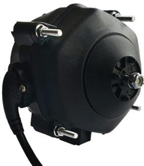
The **ECR 2** is an electronically commutated motor (ECM) that accepts input voltage from 70-264V. It can be factory programmed to three discrete speed settings from 300-1800 RPM in either direction, or with timed operations.
