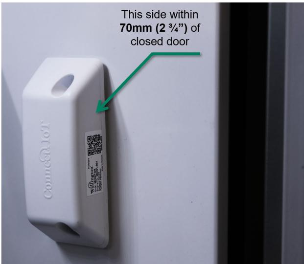
The front edge of the Connect Monitor should be installed within 70 mm (2 3/4") of the point where the door seals touch the cabinet wall.
