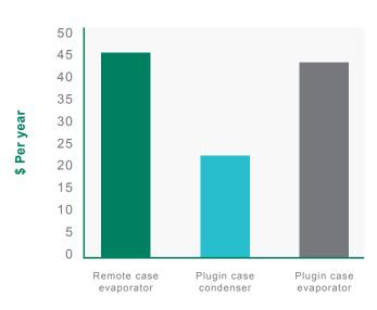
Based on \$0.11/kWh and 200/28 fan at 1550 RPM
