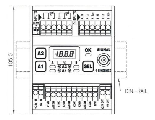
**Input:** 2 x 3 wire RTD type PT100 temperature sensor.
