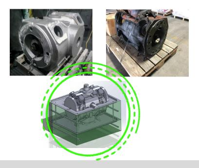
By using ExOne technology, the complex mold was ready for the casting pour in 1 week to meet the aggressive delivery and enable compressor repairs to begin
