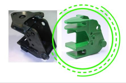
Design for Additive Manufacturing (DfAM) optimization created a one-piece component from 11 assembled parts. The speed of binder jetting the complex core enabled a final part to be delivered in under two weeks.
