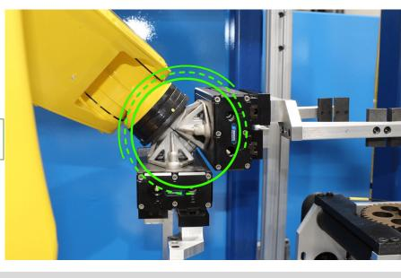
"It was one-fourth the cost of DMLS, and we did it in a strong material that reduced the payload on the robot.
