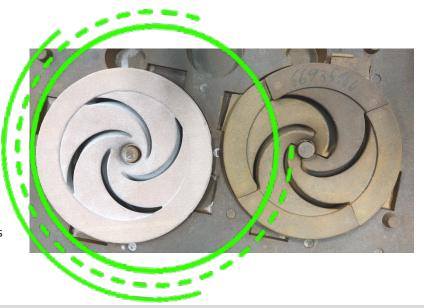
"The quality of the impeller cores has improved significantly through the 3D printing process. At the same time, the production costs have decreased by around 30%"
